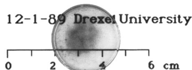
Figure 1. Representative photograph of monolithic polyacrylate-SiO 2 sol-gel glass derived from hydrosilylated poly(allyl methacrylate) (39% by mole based on the repeat unit) and tetraethoxysilane (61% by mole). The sol-gel synthesis was carried out in THF at room temperature with the molar ratios of water and HCl to TEOS being 1.53 and 0.1, respectively.
